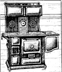
HE body and flues of Copper-Clad Ranges are not subjected to contact with rust producing damp asbestos, as is the case in all other ranges, for our pure copper lining is placed between the asbestos and heavy Allegheny Iron sheets and a dry air space is formed by a series of bosses on the copper lining, 3-16 inch in height, preserving the body and flues in a perfectly dry state. With this construction, there can be no pos sibility of the formation of rust on the inside of the
